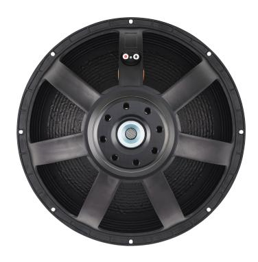
Advanced temperature control using 3-channel tuned venting system provides highly efficient cooling across the frequency band Voice coil typically operates at 30°C lower temperature than other leading drivers in this class suspension provides much greater stability and improved cone displacement symmetry
