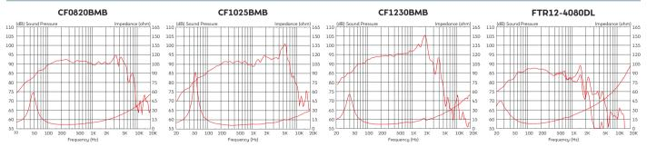
Topmost curve: Frequency response on axis | Secondary curve: Frequency response at 45° off axis | Power Rating: Tested for two hours using a continuous, band-limited pink noise signal as per AES standard.
