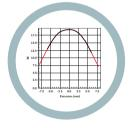
Optimised T-Pole improves cone displacement symmetry, reducing distortion
