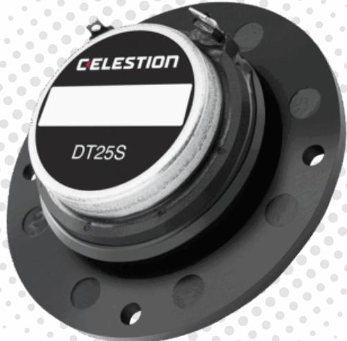
Very compact, low weight, high sensitivity tweeter 2,200Hz recommended min. crossover freq (12dB/oct) Single piece silk diaphragm and surround
