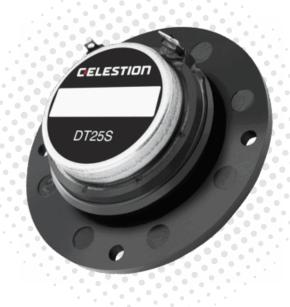
Very compact, low weight, high sensitivity tweeter 2,200Hz recommended min. crossover freq (12dB/oct) Single piece silk diaphragm and surround
