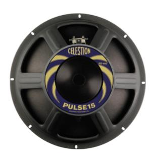
With a longer voice coil for increased 'throw' and a multi-roll surround that provides exceptional linearity and superb bass extension the 400-watt PULSE 15 is impeccably-designed sonic artillery. Featuring a Kevlar-loaded cone and rigid steel chassis designed for maximum energy transfer this robust and reliable 15 inch bass guitar speaker truly is a powerhouse of deep bass tone.
