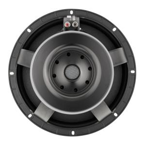
Optimised for bass and mid/bass applications Half-roll Elastomer surround enables greater Xmax/Xmech Modified T-pole enhances performance through improved BI symmetry Airflow vented magnet assembly for dynamic heat dispersion Demodulation ring for reduced harmonic and intermodulation distortion
