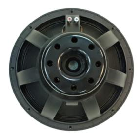
Advanced temperature control using 3-channel tuned venting system provides highly efficient cooling across the frequency band Voice coil typically operates at 30°C lower temperature than other leading drivers in this class Polysiloxane laminated double suspension provides much greater stability and improved cone displacement symmetry Lead-out wires precision woven into suspension minimises excess motion and reduces fatigue Weather resistant cone coating enhances durability
