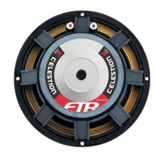
• 10in cast aluminium chassis mid/bass driver provides 400W continuous power handling and 94dB sensitivity
