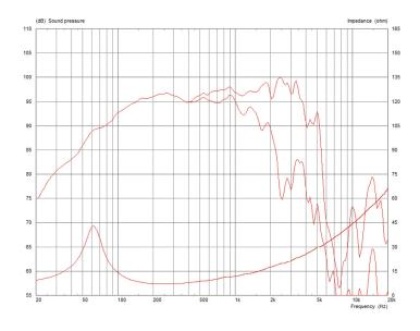
Topmost curve: Frequency response on axis | Secondary curve: Frequency response at 45° off
