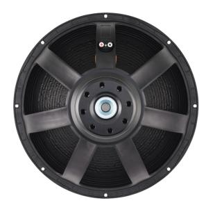
Advanced temperature control using 3-channel tuned venting system provides highly efficient cooling across the frequency band operates at 30°C lower temperature than other leading drivers in this class triple suspension provides much greater stability and improved cone displacement symmetry wires precision woven into suspension minimises excess motion and reduces fatigue weatherproof cone coating enhances durability Entures href="https://celestion.com/ten-key-
