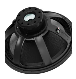
Advanced temperature control using 3-channel tuned venting system provides highly efficient cooling across the frequency band Voice coil typically operates at up to 80°C lower temperature than other leading drivers in this class Polysiloxane laminated double suspension provides much greater stability and improved cone displacement symmetry Lead-out wires precision woven into suspension minimises excess motion and reduces fatigue Double-sided, weatherproof cone coating enhances durability
