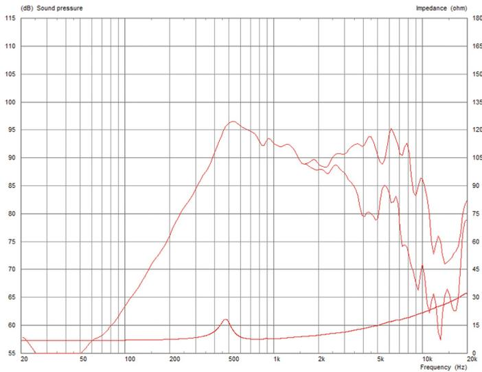
Topmost curve: Frequency response on axis |
