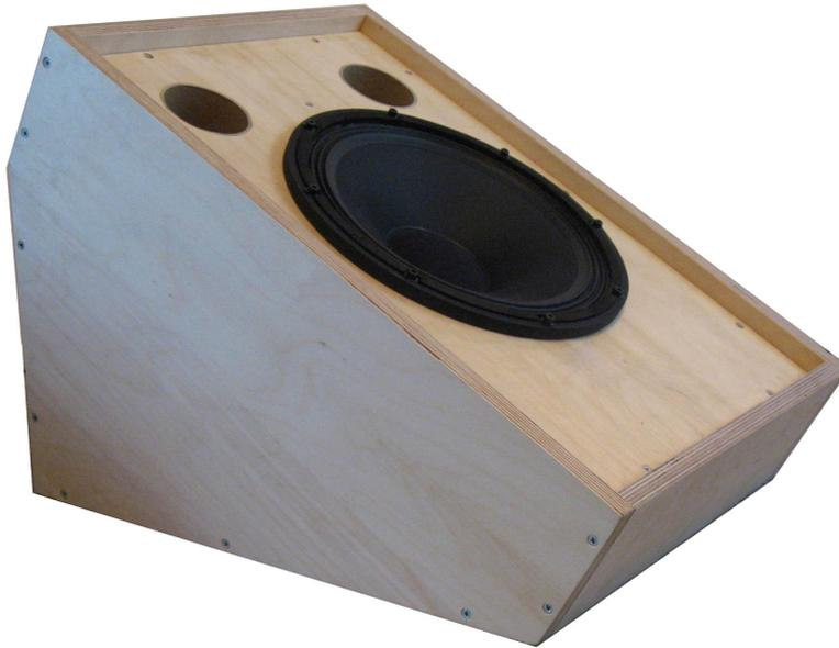
The CKT-FM-FTX1225 system is a medium sized 2-way coaxial floor monitor. This system is based around the 12"(300mm) FTX1225. The coaxial arrangement of the bass and treble drivers provides wide and uniform dispersion in both horizontal and vertical planes ensuring a clear and balanced sound over a wide area. The compact and portable cabinet allows for mounting with the driver axis at 30 or 60 degrees up from the horizontal.
