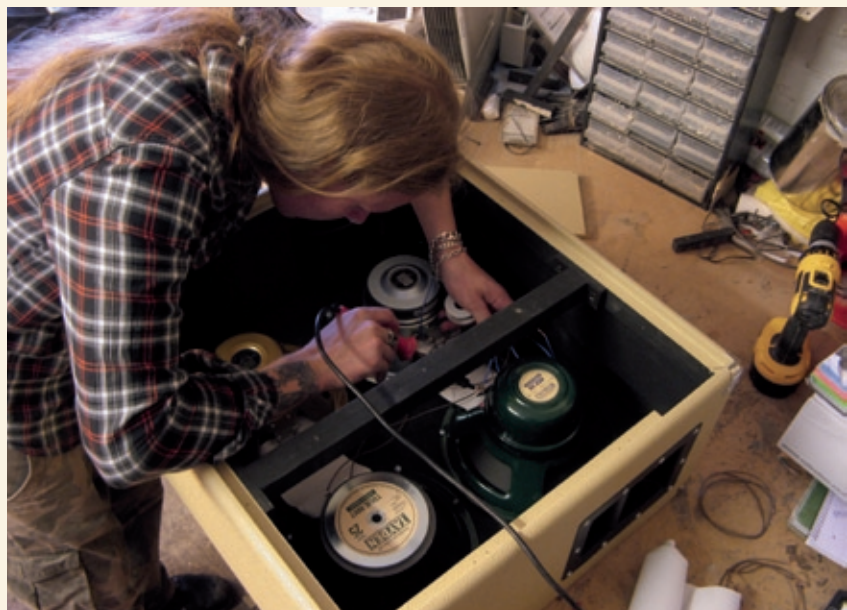
Paul Gough of Zilla assembles the special 4x10 cabinet described in this feature. The Tayden speaker visible in the photo unfortunately turned out to be defective, hence the eventual all-Celestion lineup.
