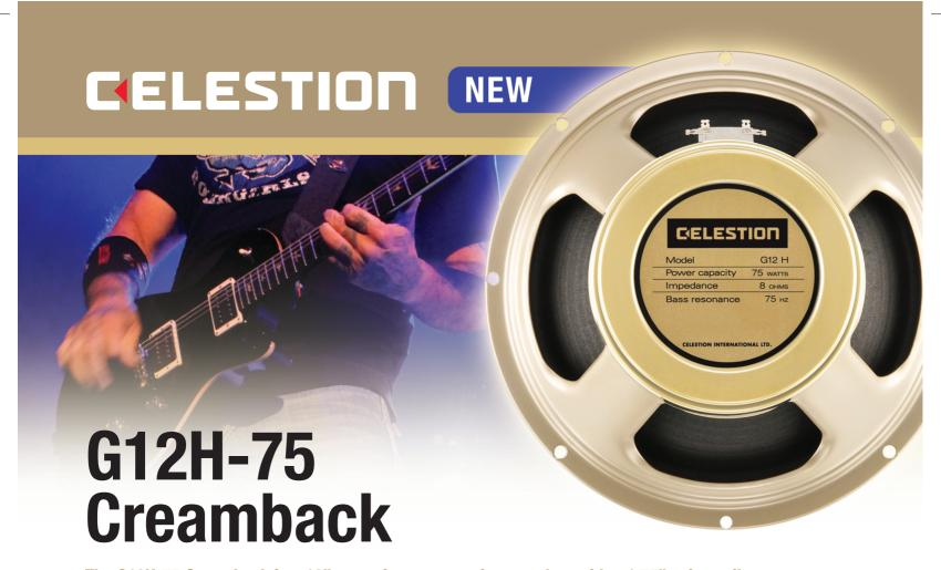
The G12H-75 Creamback is a 12" ceramic magnet guitar speaker, with a 1.75" voice coil, offering 100dB sensitivity and 75-watt power handling with true vintage tone.
