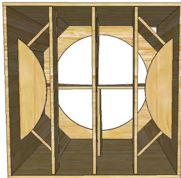
Back braces installed
