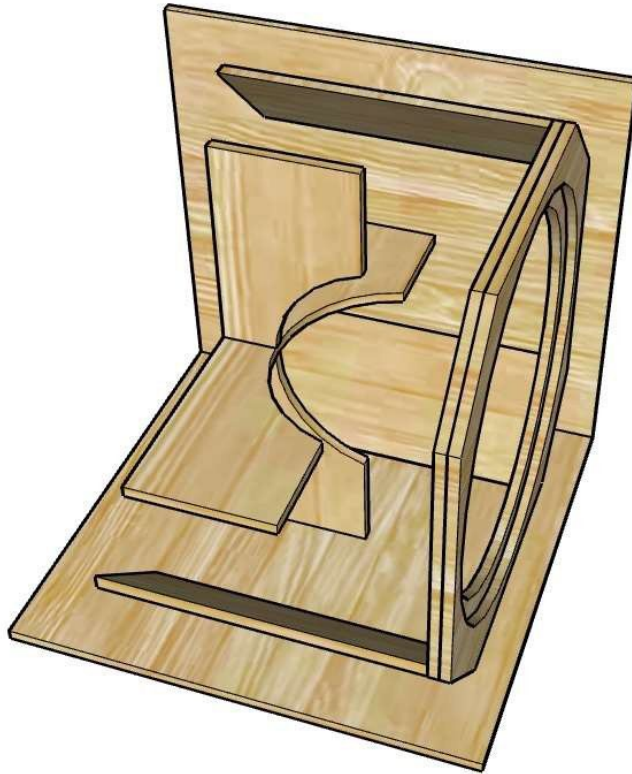
Side, top and bottom braces installed, 'X-ray' view
